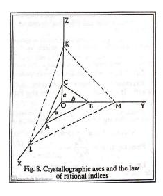
Let OX, OY and OZ represent the three crystallographic axes and let ABC be a unit plane. The unit intercepts will then be a, b and c. Accordingly the intercept of any face such as KLM, on the same three axes will be simple whole number multiple of a, b and c respectively.
